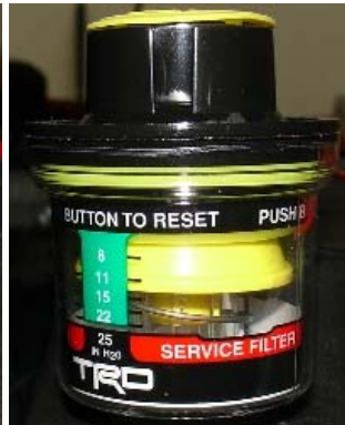
Partially Dirty Filter (Do Not Clean Now)
