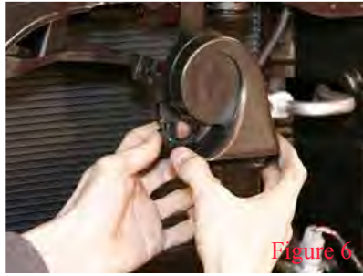
Optional Step: Remove both horns by unclipping the wiring harness and then remove the stock bolt holding in place. This will allow you more room to work.
